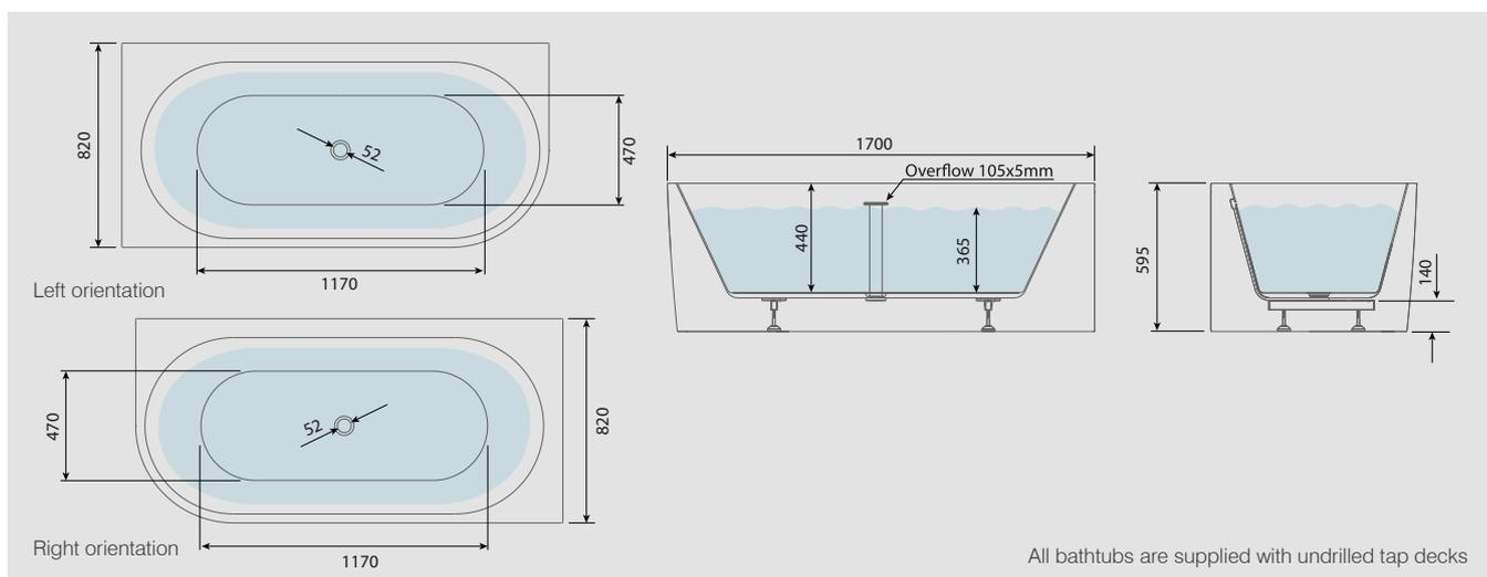
All bathtubs are supplied with undrilled tap decks
