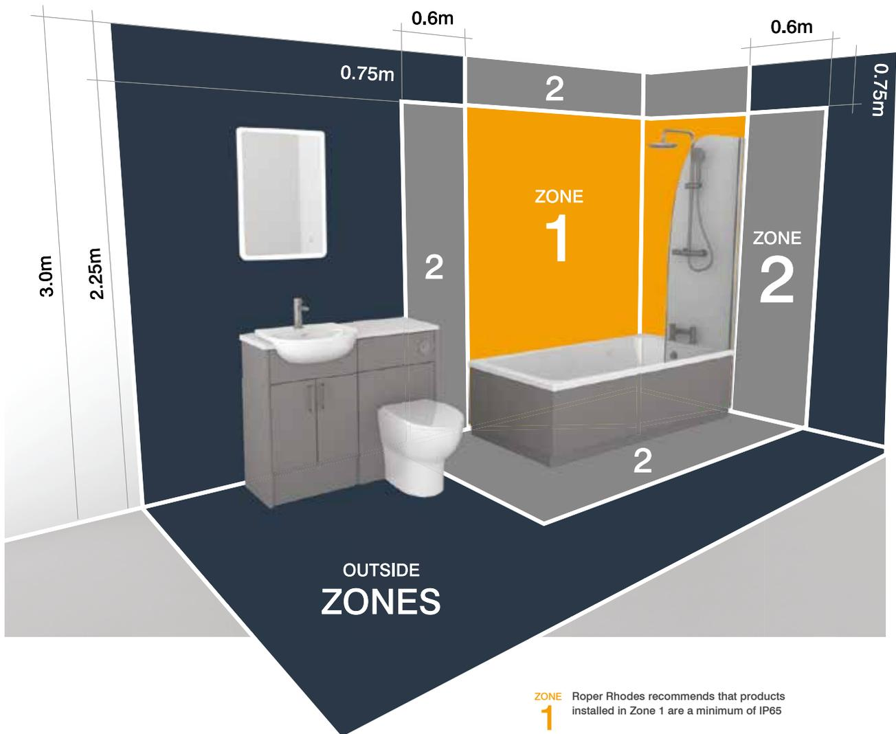
**ZONE 1** Roper Rhodes recommends that products installed in Zone 1 are a minimum of IP65
