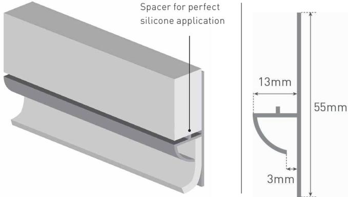
Our new PVC floor to wall profile gives a neat and accurate finish to vinyl floor and wall fittings. Easy to cut and fit, this trim allows the vinyl flooring to be changed without having to replace any of the panels. The ridge spacer provides the perfect gap for silicone sealant and the vinyl flooring can be fixed securely under the flap at the base of the trim.
