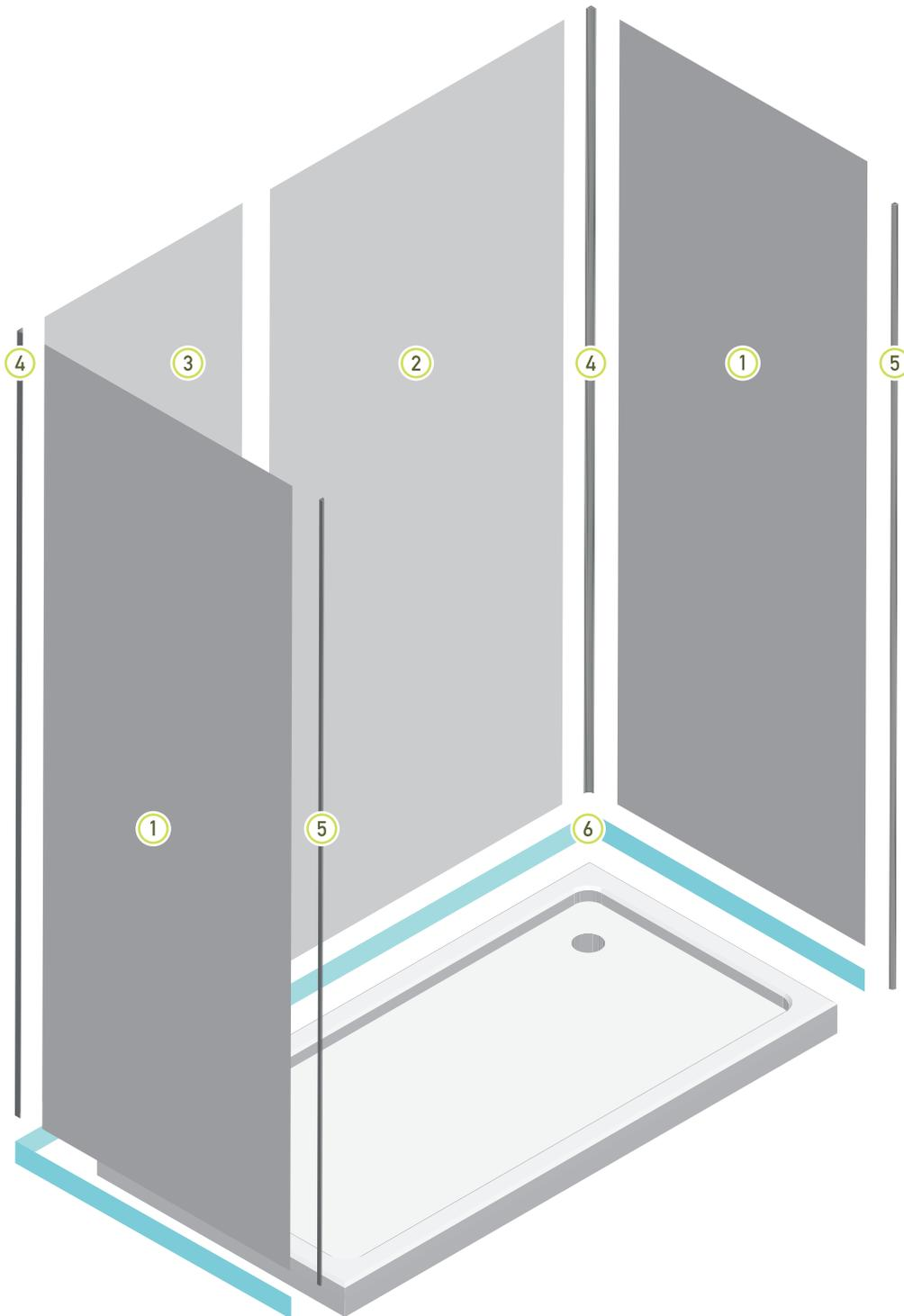
The above illustration shows a typical installation of a 1800mm x 900mm shower enclosure
