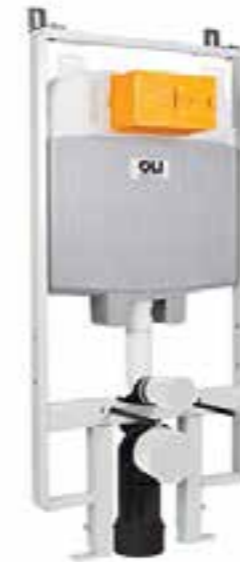
1200cm Slim Pre-wall, freestanding w.c. frame including brackets and w.c bend with 3/6 litre dual flush plate front flush installation only.
