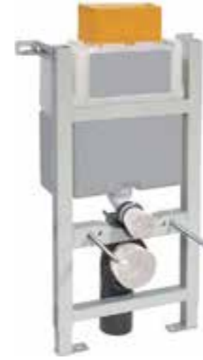
820cm Pre-wall, freestanding w.c. frame including brackets and w.c bend with 3/6 litre dual flush plate top or front flush installation.
