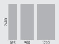
Hydrolock® panels are available in a range of widths for ease of installation;
